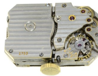
14 - The movement of the Tiffany's watch in picture 13, Angelus SF-N 9.
